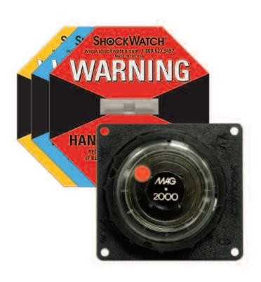
ShockWatch Impact Indicators detect and record impact and mishandling of fragile, sensitive, or calibrated products during transportation.
