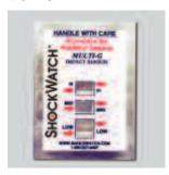
A version of the clip product, the Multi-G houses three tube sensitivities in a single unit. It is designed for determining package sensitivity during drop testing.
