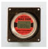
Economical, resettable, and tamper-proof, this impact detection device can be used for large crates and shipments over 100 lbs., and also records the date and time of an impact.
